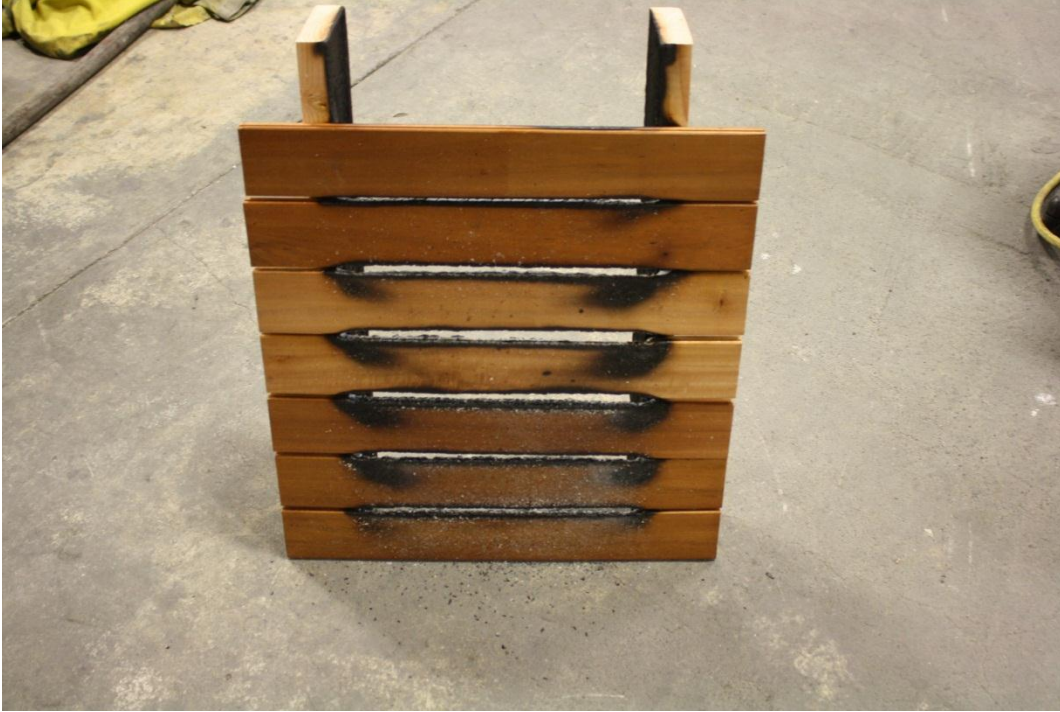
Deck surface post test
